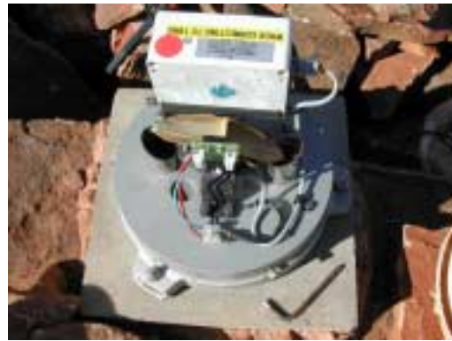
The inside workings of a pluviometer showing tipping-buckets, Sambot Pluvio; Photographer: Rob Kelman
