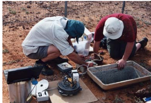
Servicing a pluviometer
