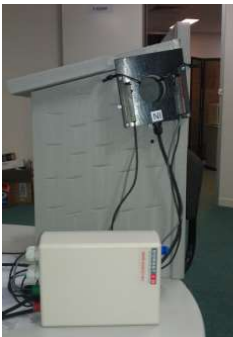
“In-Out” optical beam sensors on a Trovan circular 50mm diameter antenna used to monitor Leadbeater’s Possums in and out of an artificial fire-proof nest box
