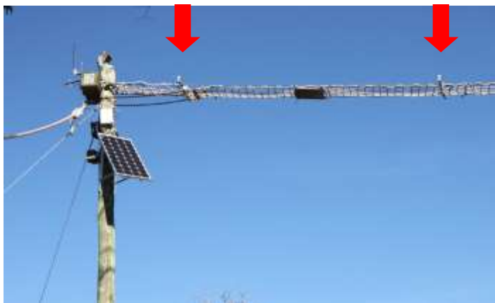
Single optical beam sensors (arrowed) sited either side of a Trovan flat panel square antenna on a rope bridge used for monitoring possums and gliders crossing the Hume Highway
