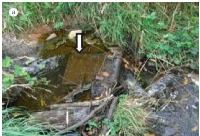
Semi-submerged large “pipe” antennas to monitor platypus in a stream in Tasmania
