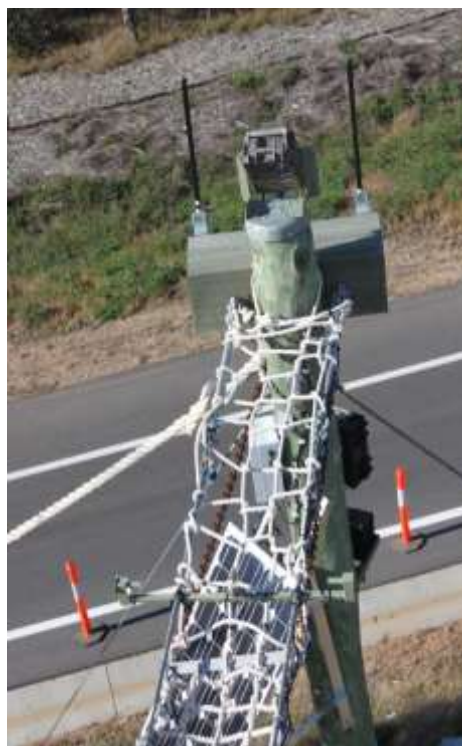
4G mobile phone network modems are used to transmit data from these rope bridge monitoring systems on the Hume Highway in NSW to researchers in Melbourne
