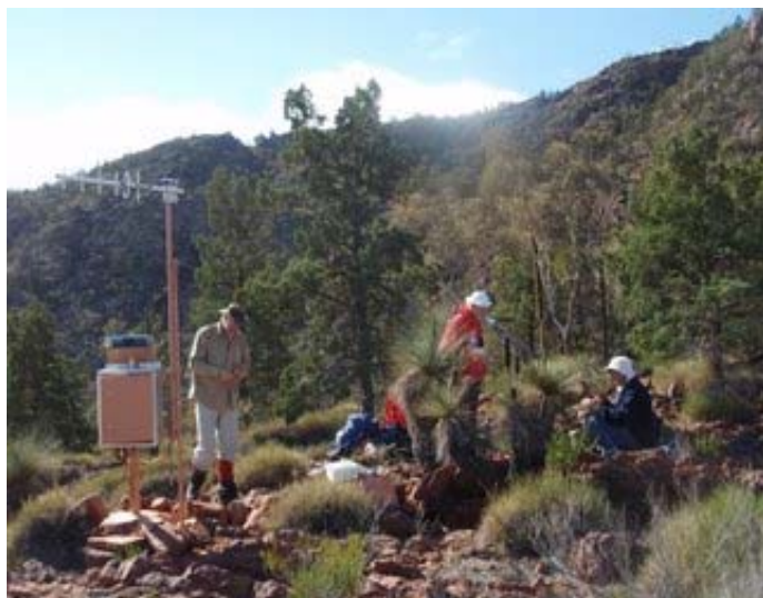
Figure 6: The Modem box which contains the telemetry equipment at Arcoona Bluff, a Yagi antenna is used to send the signal to Mt Scott Repeater at Leigh Creek.
