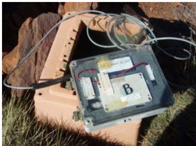
Figure 5: The old HS logger "B" inside the larger sealed box. The Battery pack is installed just above, and will last for 3 years without needing a change.
