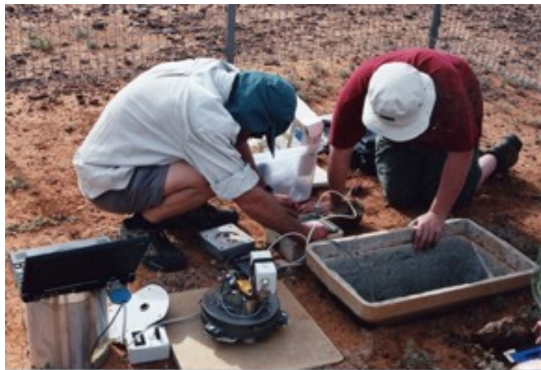
Servicing a pluviometer
