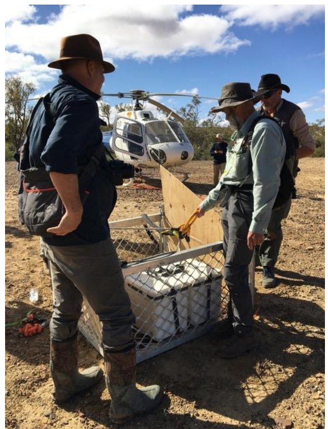
Aerated fish carrier in a cradle to be lifted by helicopter. The cradle includes stabilising fins to prevent it spinning while being transported. Photo A. Vincent
